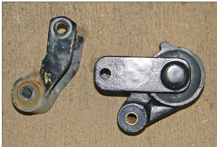
Factory shackle and Sulastic torsion shackle.
