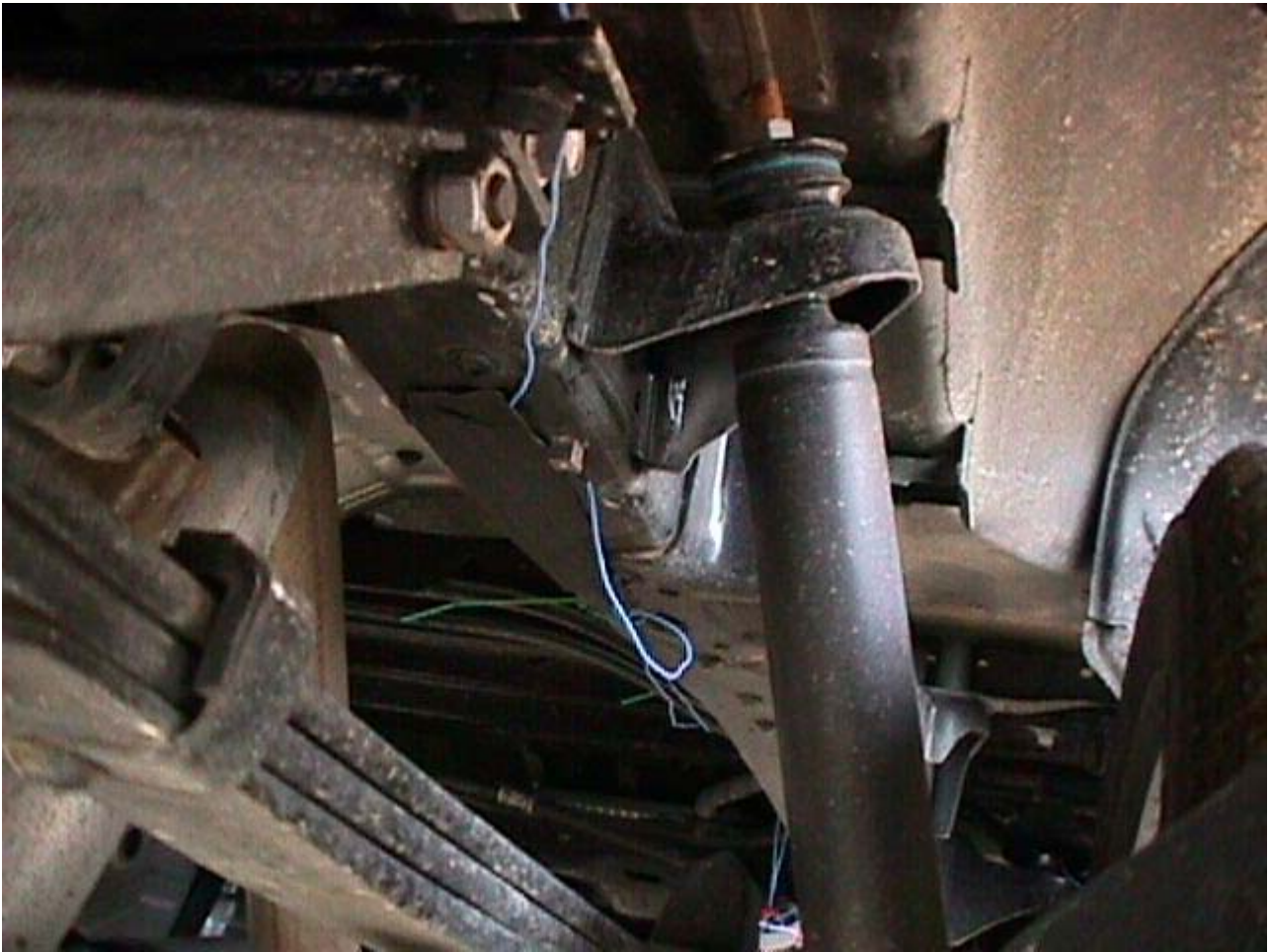
Triaxial Accelerometer #2 at right shock tower
