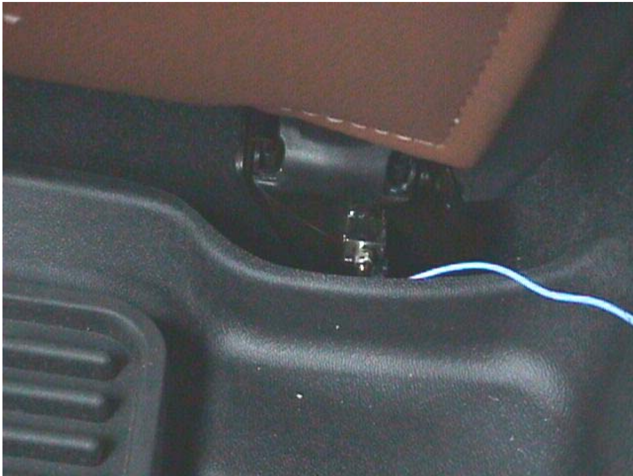
Triaxial Accelerometer #6 on drivers right rear seat pedestal
