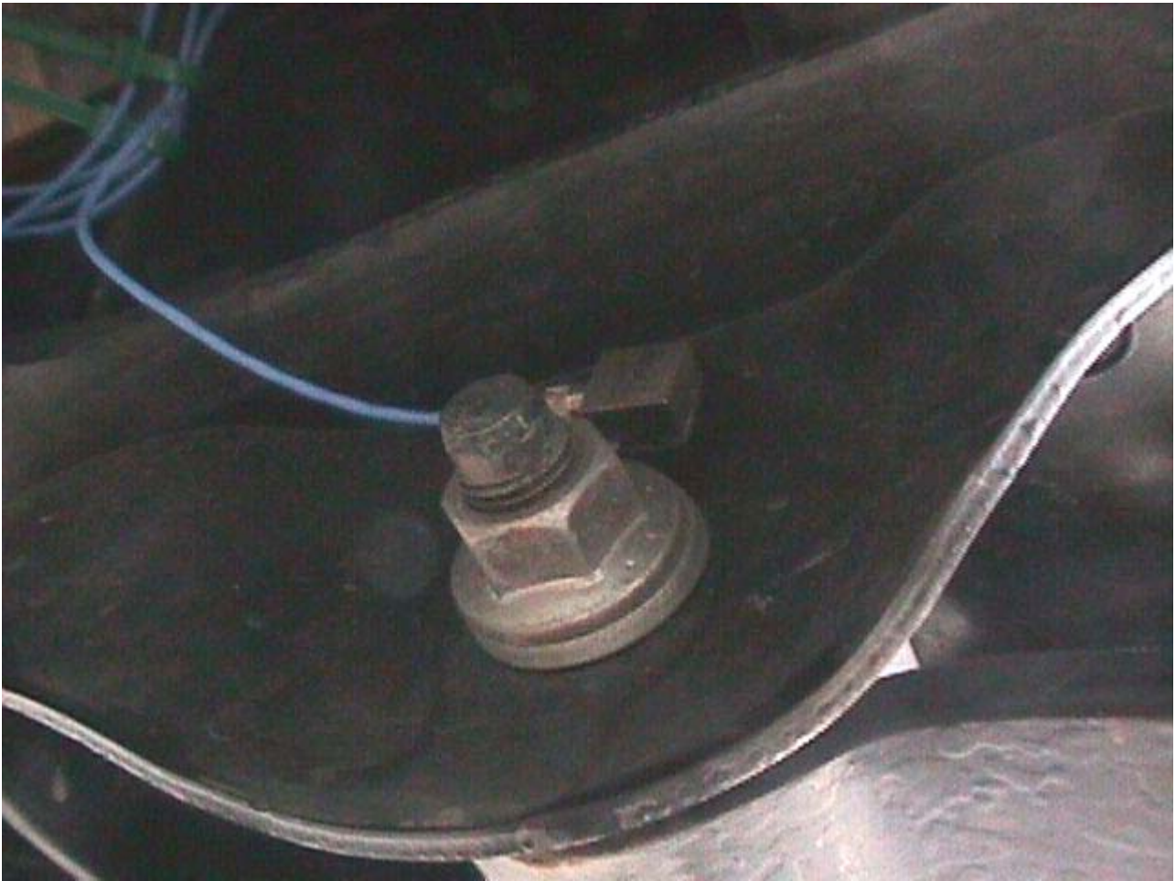
Triaxial Accelerometer #3 at front spring eye
